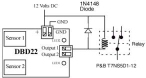
The DBD22 can drive a relay with a low current coil. The relay shown has a coil current of 30 ma and a contact rating of 10 amps (Digikey PB380-ND). A clamping diode is required when driving a relay to suppress the voltage spike
