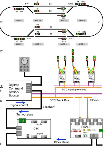
A loop like this is probably not what you want to signal. However, we suggest you connect enough items (CSCe, SHD2, signal heads and block detectors) to your system to verify operation before making any changes to the CSCe.
