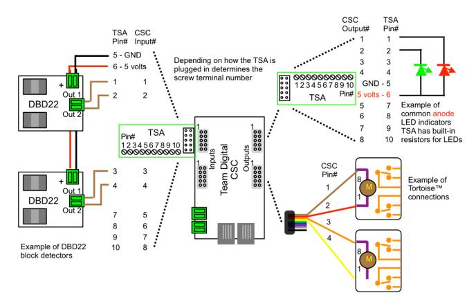
Additional example of input wiring. Inputs can be used for DBD22s, turnout feedback from switch machines and push button control of turnouts as shown or for connection to turnout contacts for turnout feedback.
