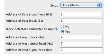
**Block detectors connected to inputs?:** Will DBD22 block detectors be connected to the CSCe inputs. If yes, then input one is assigned to the first block (B1). Connect the DBD22 output used for BI to input one. Connect the other detectors to inputs in sequential order. If no, then the CSCe will expect to receive block status over the serial bus.
