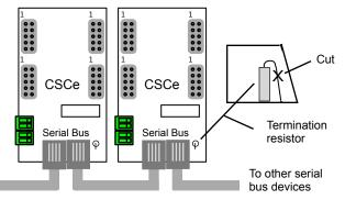
In a systems when more than 10 Team Digital products are connected to the serial bus, the bus terminating resistor should be cut on any additional devices.
