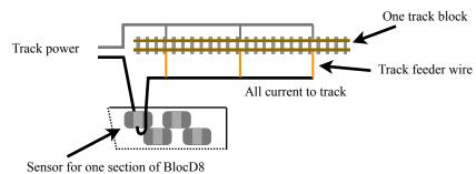
Locomotives, lighted cars and rolling stock with resistive wheels sets draw different amounts of current from the track. The BlocD8 has two potentiometers to adjust sensitivity. Turning the pot CCW will increase the sensitivity. **If the pot is turned fully CCW there may be false block detection**. Passing the feed wire through each sensor two times will increase the sensitivity and can improve reliable detection. See "TIP" in section 2.
