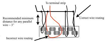
The diagram shows correct and incorrect ways to route wires. Incorrect routing of wires will cause false block detection. Wires with DCC current should be routed away from the sensors in a perpendicular manner.
